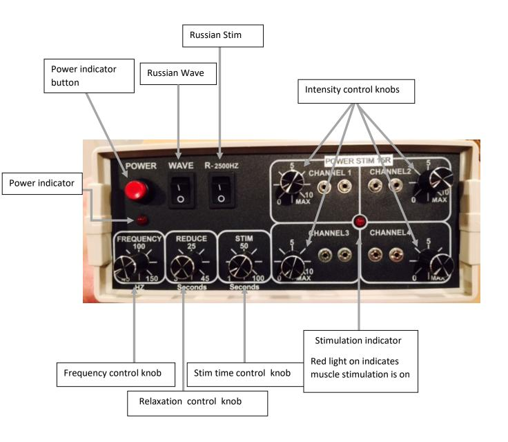
The PowerStim 15R has 4x Intensity Control Knobs, 3x System Control Buttons, 3x Pulse Control Knobs, and 2x Red Light Indicators. Below is a description of the functionality of each of these controls.
